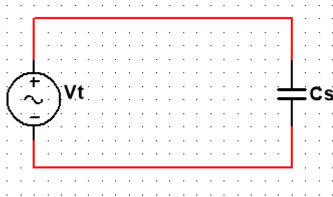
Figure 1. Equivalent most basic circuit for dielectric spectrometer analysis.
