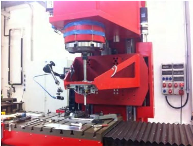
Figure 2. Friction Stir Processing equipment.
