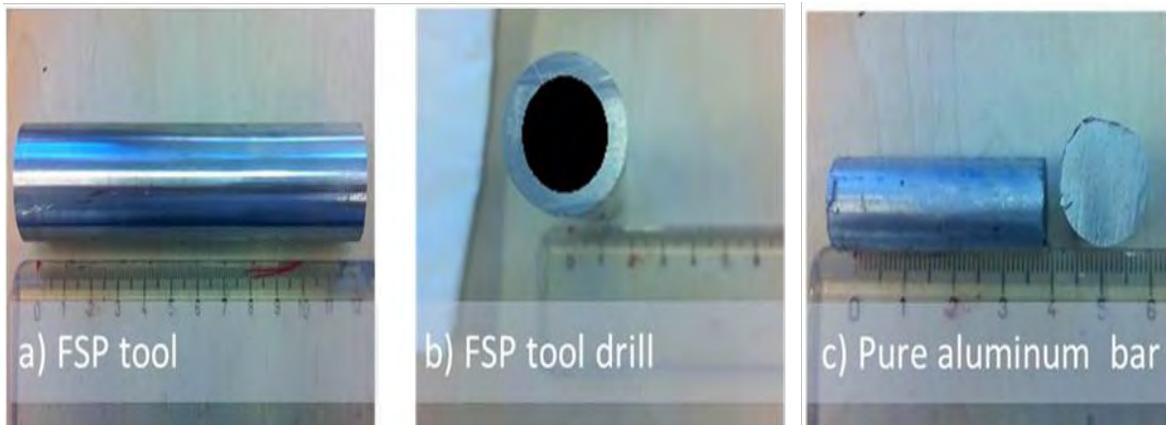
Figure 1. FSP tool system.
