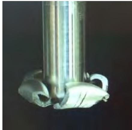
Figure 4. FSP tool system rupture.
