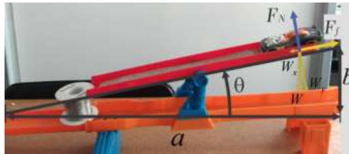
Figure 7. Experimental setup used to calculate the friction angle and the coefficient of friction.
