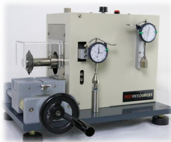
Figura 3 Muescadora V Shaped Notch Maker. V 402V (TestResources, 2016).
