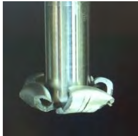
Figure 4. FSP tool system rupture.
