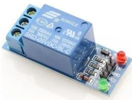
Figura 1.3 Modulo relee o relay
