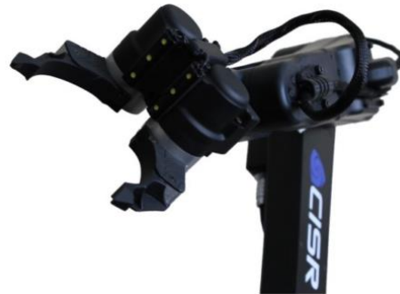
Figura 5 (a) Pinza robótica háptica. (Nahavandi, Mullins, Fielding, Abdi, & Najdovski, 2015)
