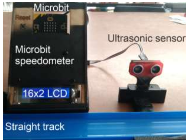
Figure 5. a) Speed measurement unit conformed by a micro:bit, a micro:bit expansion board, a 16x2 LCD and an ultrasonic sensor.
