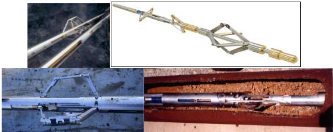
Figura 1. a) MaxTrac PSTT. b) Tractor MDT001. c) Understanding Downhole. d) MDT Downhole Tractor.
