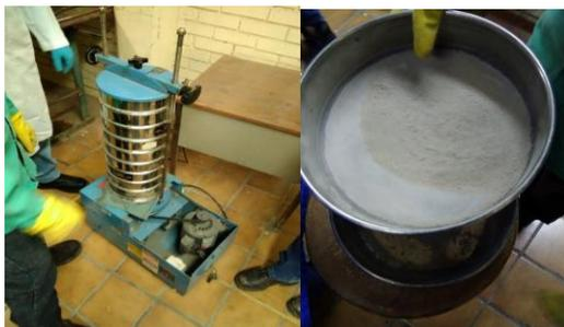
Figura 2. Tamiz ROTAP y mineral cribado
