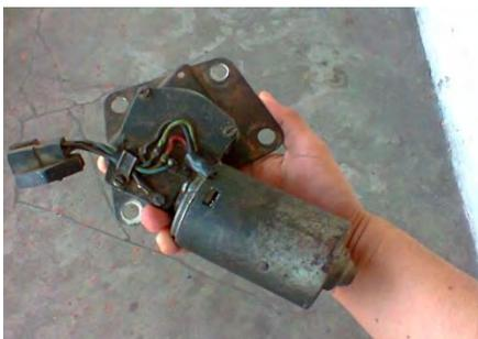
Figura 21: Motor reductor.
