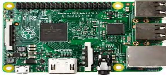
Figura 1. Raspberry Pi 2 Modelo B (*Uk.rs-online.com*, 2016)
