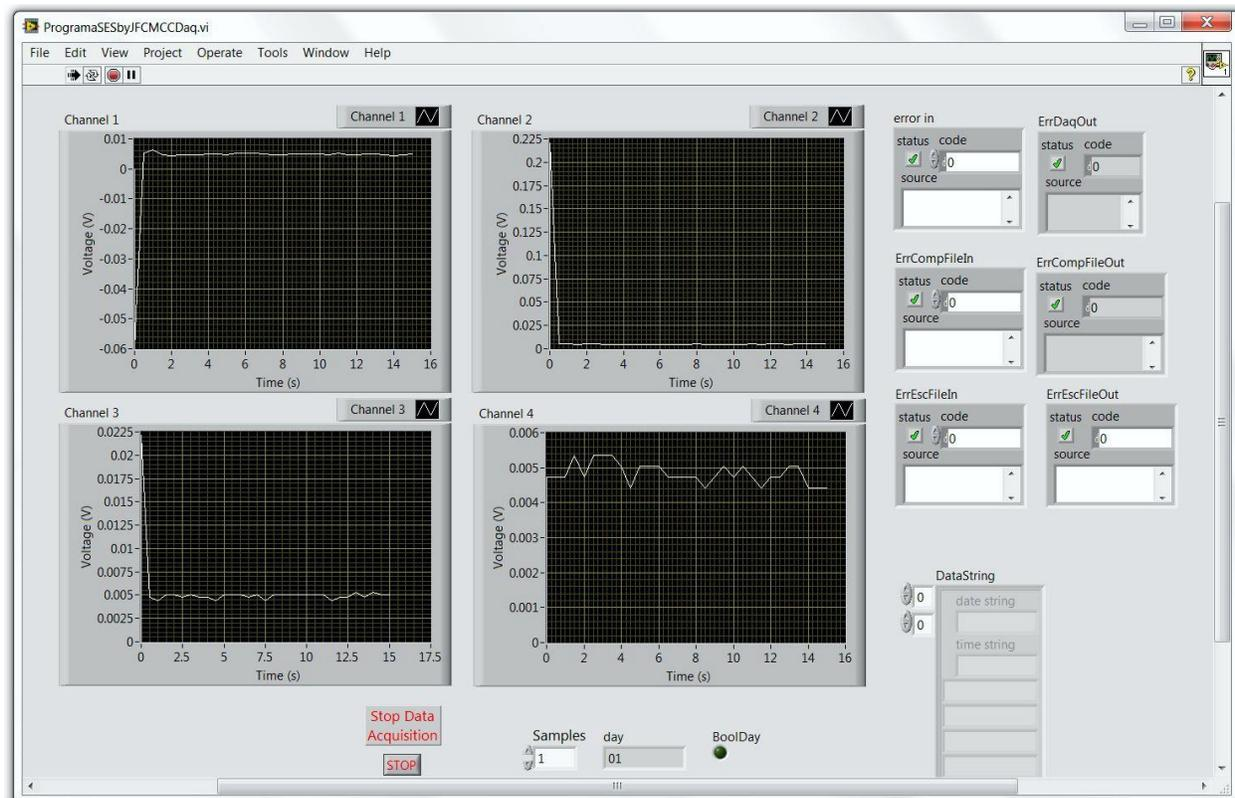
Figure 2. Main window of the LabVIEW program to measure the geoelectrical signals.
