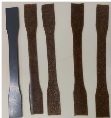
Figure 6. Specimens cut from the adapted synthesis.
